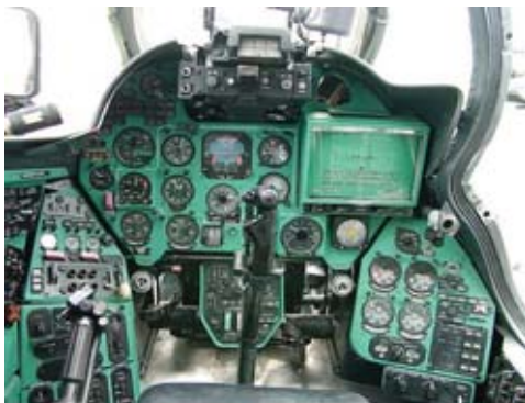
Fig. 2. The cockpit with components of the communication system in use until now (left) and the ITWL-developed integrated communication system ZSL-1 (right) built into the Mi-24 helicopter
